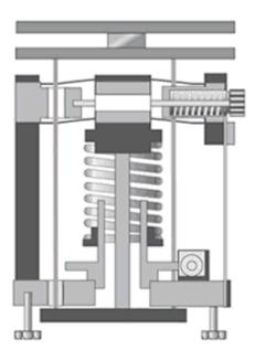
While effective isolation from both air and ground borne vibrational energy is important throughout the audio playback chain, it is essential for vinyl playback. It can be built into a turntable in the form of spring or "O" ring suspensions but current thinking downplays that in favor of separate isolation stands rather than incorporating it into the turntable itself.
