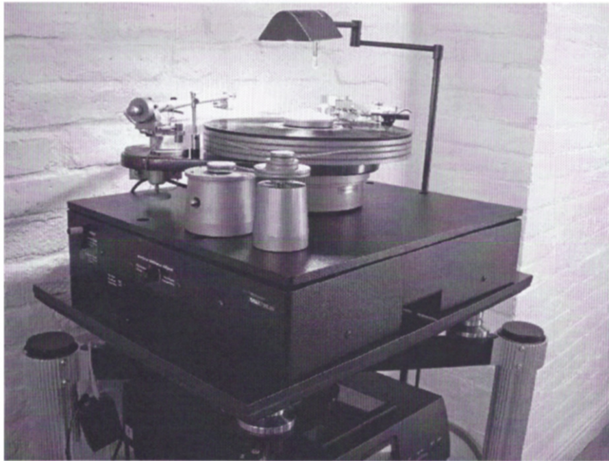
Figure 4 A Simon Yorke vinyl-record turntable on the Minus K BM-8 vibration isolation platform to ensure extra high-fidelity sound quality
