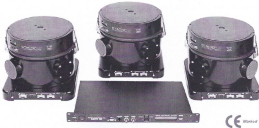
Figure 5 STACIS active piezoelectric vibration control systems from Technical Manufacturing Corporation use inertial vibration sensors and piezoelectric actuators to cancel vibrations from 0.6 Hz upwards with an active bandwidth of 250 Hz
