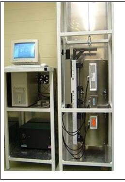
*Conventional vertical Bridgman furnace use to grow the semiconductor material cadmium zinc telluride (CZT).*
