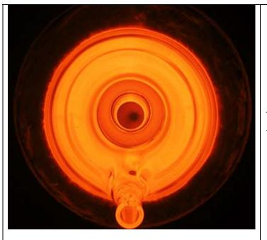
*Looking down a quartz-lined furnace at 1100° C.*
