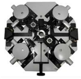
The MicroView4000 platform from Nanonics Imaging is the basis for AFM-Raman integration.
