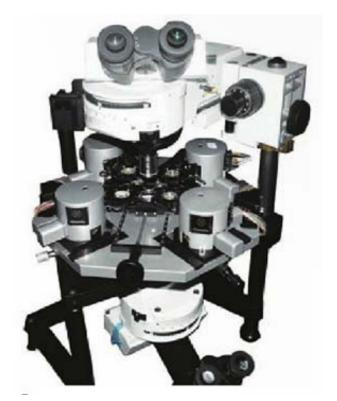
Nanonics MultiView 4000 MultiProbe System for scanning probe microscopy permits full integration with optical techniques such as Raman using Negative-Stiffness vibration isolation.
