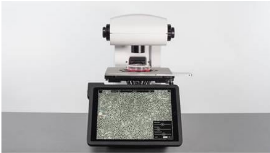
Revolve combines the full functionality of both upright and inverted microscopes.
