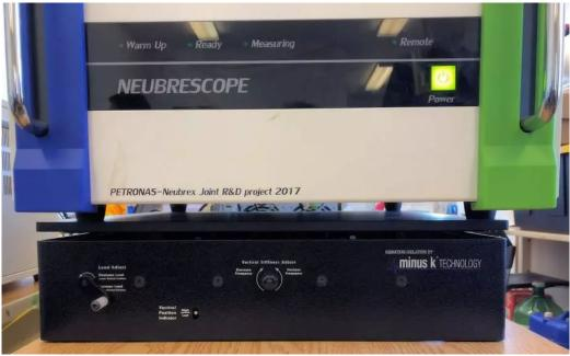
Negative-stiffness vibration isolator beneath the Neubrescope.
