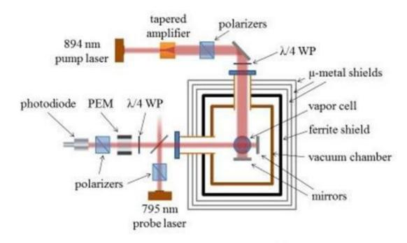
Diagram of the co-magnetometer in position at the South Pole.
