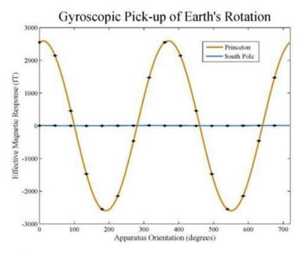
Comparision of the gyroscopic pick-up of the Earth's rotation measured in Princeton and at the South Pole.
