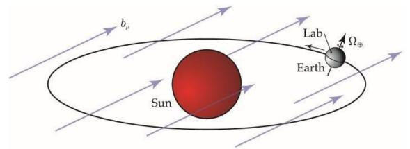
The Romalis Group uses ultra-high precision techniques involving polarized atomic spin to test Lorentz symmetry. The presence of Lorentz violation would appear as an effective field felt by the atoms. Presumably, this field acts as a cosmically fixed background which, from the point of view of our Earth bound experiment, fluctuates with a sidereal period as the Earth rotates in it.
