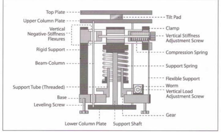
Negative stiffness vibration isolation technology offers transmissibility advantages at multiple frequencies compared with high performance air tables. Source: Minus K Technology Inc.
