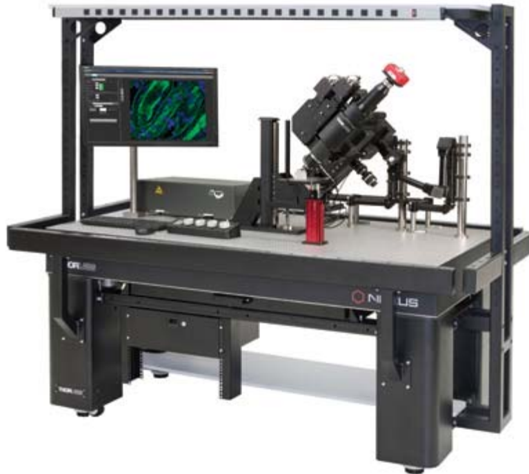
FIGURE 2. A Thorlabs optical table and workstation is shown supporting the Thorlabs Pergamon II Series multiphoton microscope system, a femtosecond-laser source, and a computer. ( Courtesy of Thorlabs )
