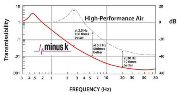
Laser-based interferometers are extremely sensitive devices that are capable of resolving nanometre scale motions and features. They often have very long mechanical paths, which makes them even more sensitive to vibrations. The sophisticated modern ellipsometry techniques that allow this high performance rely on low noise to be able to detect fringe movement. Properly isolating an interferometer will allow it to provide the highest possible resolution.
