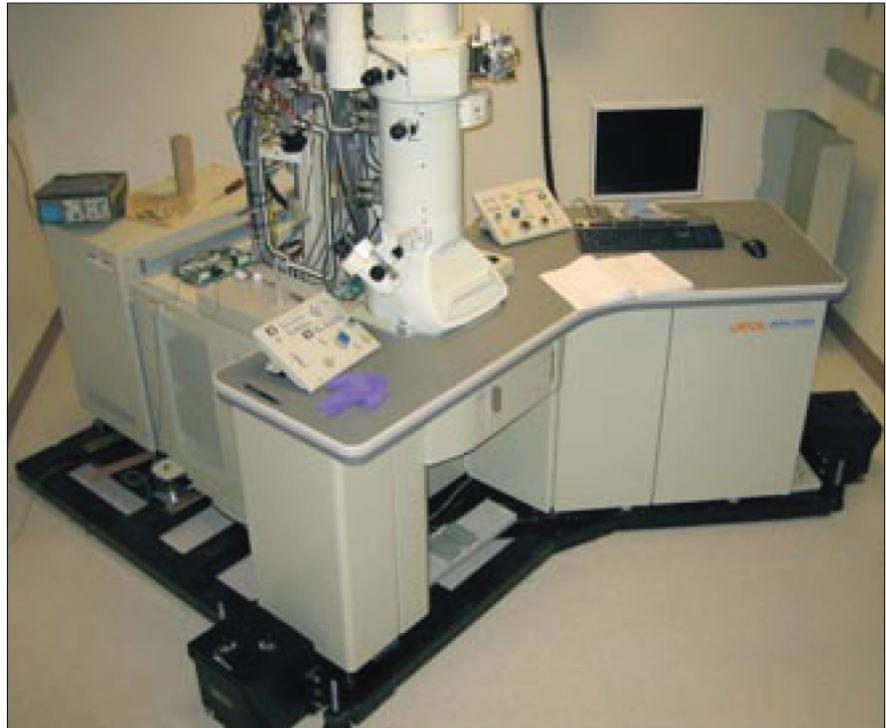
CLM's JEOL 1400-transmission electron microscope positioned on negative-stiffness isolators.
