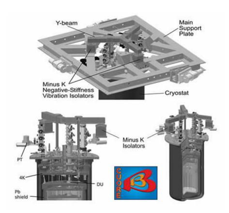
Italy's National Institute of Nuclear Physics (INFN) has installed three custom vibration isolators for experiments within the Cryogenic Underground Observatory for Rare Events (CUORE), located within Gran Sasso mountain, the highest peak in the Apennines about 100 km (62 miles) from Rome.
