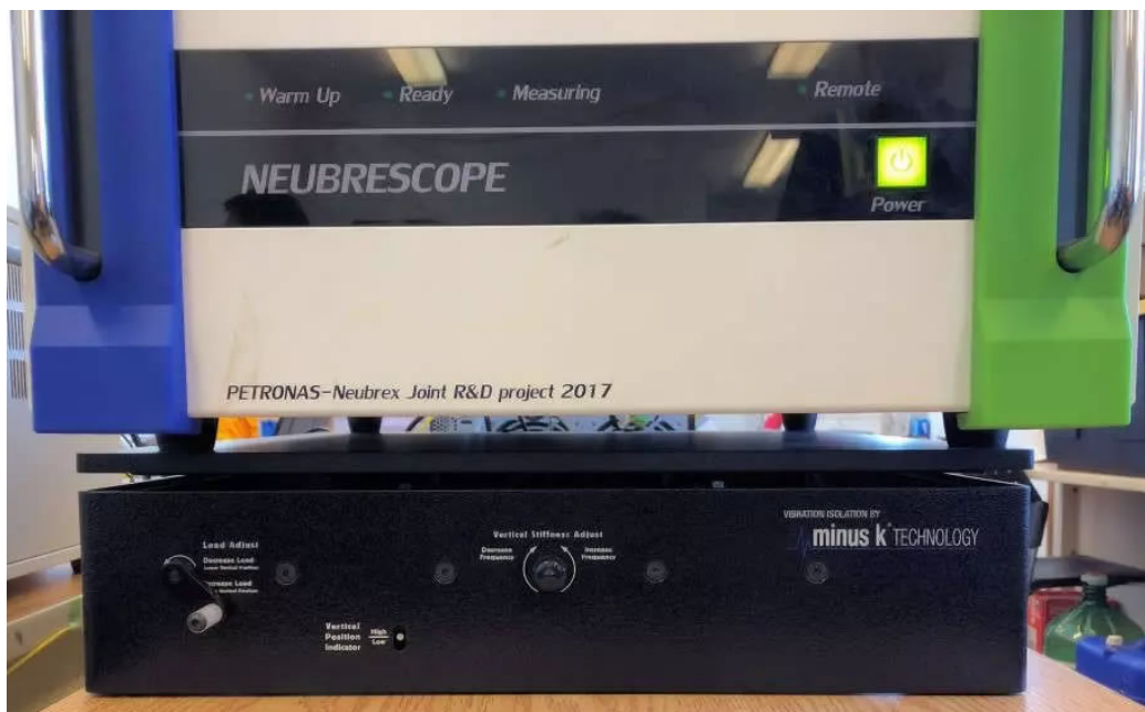
Negative-stiffness vibration isolator beneath the Neubrescope.
