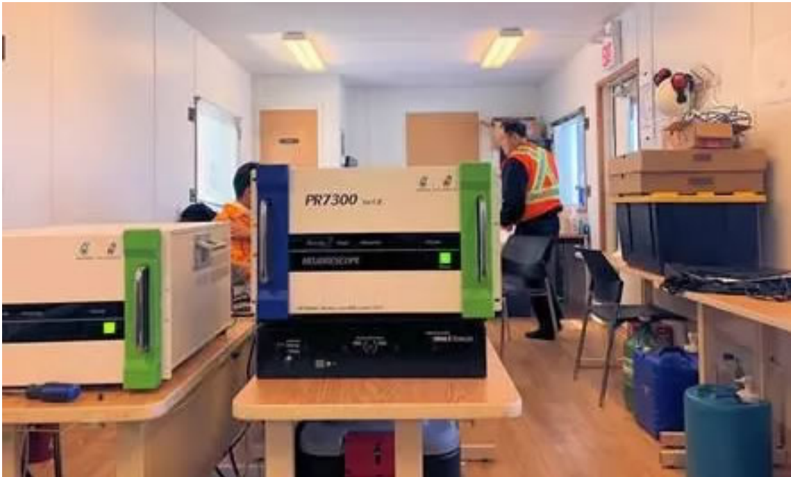
Neubrescope positioned on a negative-stiffness vibration isolator at the Neubrex well-site facility.
