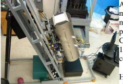
At the SMART Laboratory, crystals of CdZnTe and the scintillator materials are grown via a vertical Bridgman furnace. In this process, molten material is directionally solidified from one end to the other to produce a large-volume ingot that is a single crystal. Methods to grow CdZnTe for gamma-ray spectrometers have been explored since the early 1990s, yet a reliable system to produce large crystals at an economical cost has not been achieved until relatively recently.
