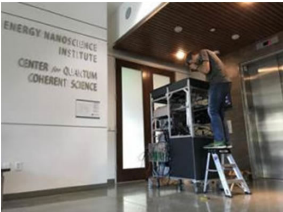
miniG transportable, multi-axis atom interferometer, currently in development by UC Berkeley's Müller Group. (Courtesy Müller Group)
