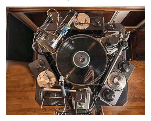
The turntable's 3 drive pods, each with 2 synchronous motors, drive a15 lb. flywheel.
