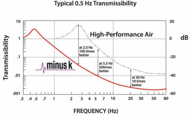
Negative-stiffness isolators employ a completely mechanical concept, with no air or electricity required. There are no motors, pumps or chambers, and no maintenance because there is nothing to wear out and they operate purely in a passive mechanical mode. Vertical-motion isolation is provided by a stiff spring that supports a weight load, combined with a Negative-Stiffness mechanism.
