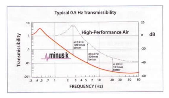
Negative-stiffness isolators resonate at 0.5 Hz. At this frequency there is almost no energy present. It would be very unusual to find a significant vibration at 0.5 Hz. Vibrations with frequencies above 0.7 Hz (where negative-stiffness isolators begin isolating) are rapidly attenuated with increase in frequency.
