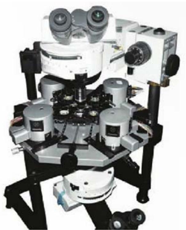
Nanonics MultiView 4000 MultiProbe System for scanning probe microscopy permits full integration with optical techniques such as Raman using Negative-Stiffness vibration isolation.
