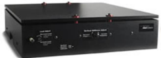
the "beam-column" effect. A beam-column behaves as a spring combined with a NSM. The result is a compact passive isolator capable of very low vertical and horizontal natural frequencies and very high internal structural frequencies.
