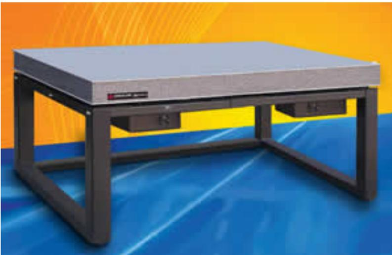
Minus K Technology, a leading manufacturer of vibration isolation products has partnered with Kinetic Systems, Inc in designing a new, versatile, ultra-low-natural-frequency optical table isolation system. The MK52 negative-stiffness optical table achieves 0.5 Hz or lower vertical and horizontal natural frequencies without limiting its ability to support static loads. When adjusted to a 0.5 Hz natural frequency, the MK52 achieves 93% isolation efficiency at 2 Hz, 99% at 5 Hz, and 99.7% at 10 Hz.
