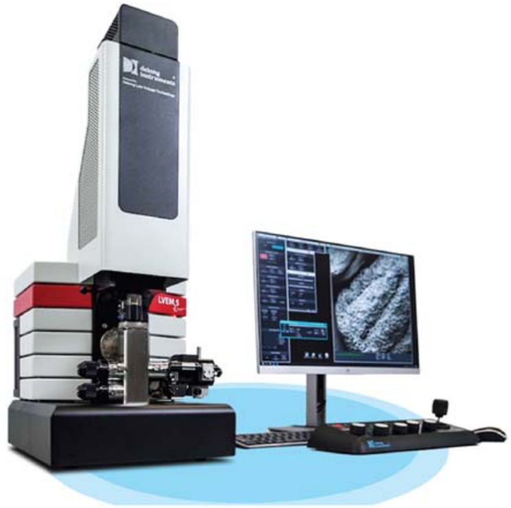
Figure 1: LVEM5 benchtop electron microscope combines high-resolution imaging with nanoscale resolving power. (Image courtesy of Delong America.)
