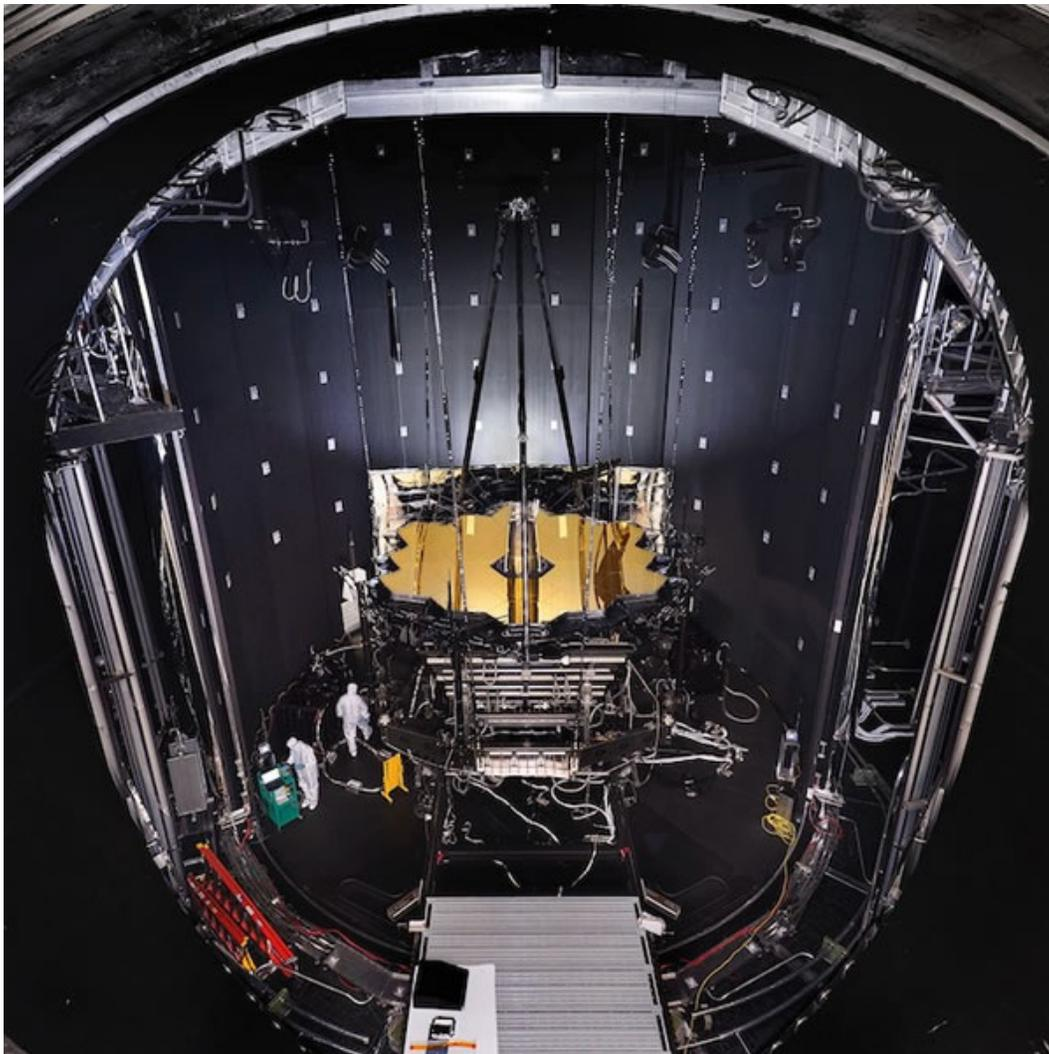
NASA's James Webb Space Telescope suspended from the Minus K vibration isolators on top of Chamber A at NASA's Johnson Space Center in Houston. (Courtesy of NASA/Chris Gunn)
