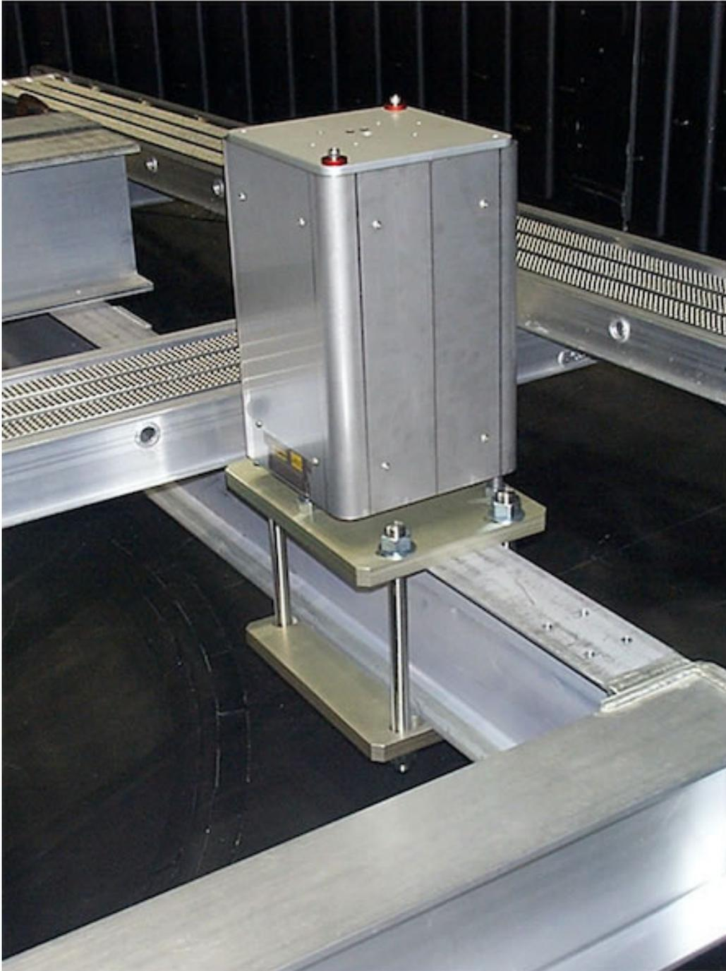
One of three Negative- Stiffness vibration isolators used on the Cryogenic Telescope Assembly, Spitzer Space Telescope.
