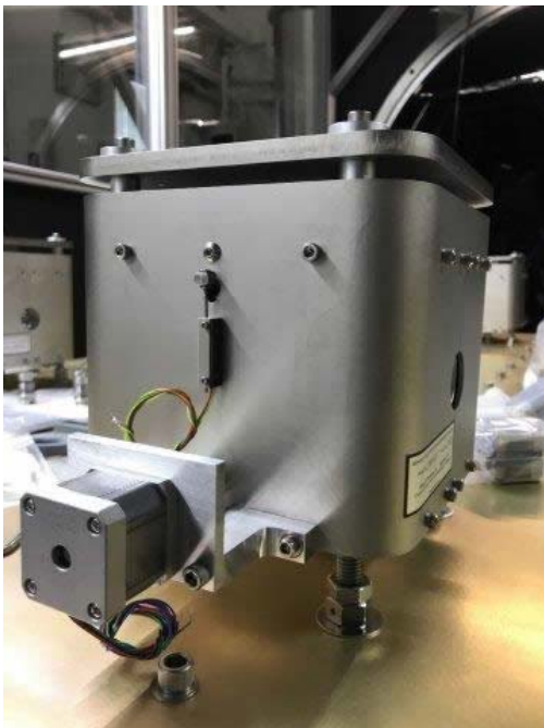
One of the five 800CM-1CV Negative-Stiffness isolators supporting the Keck Planet Finder. (Courtesy UC Berkeley Space Sciences Laboratory)
