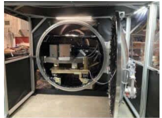
Optical components of KPF are positioned on a bench inside a vacuum chamber. (Courtesy UC Berkeley Space Sciences Laboratory)
