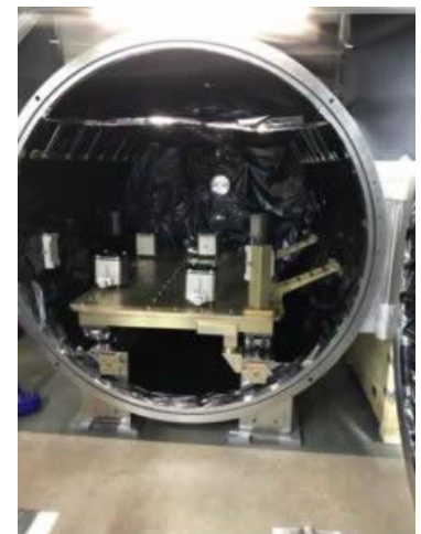
Negative-Stiffness isolators in position within the KPF. (Courtesy UC Berkeley Space Sciences Laboratory)
