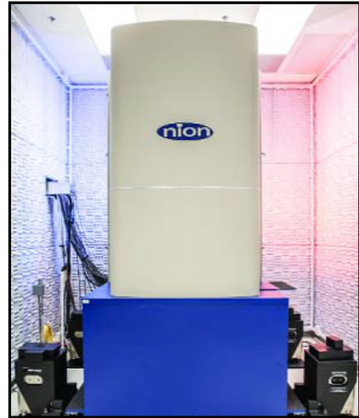
IMRI’s Nion UltraSTEM 200 positioned on a Negative-Stiffness vibration isolation floor platform.
