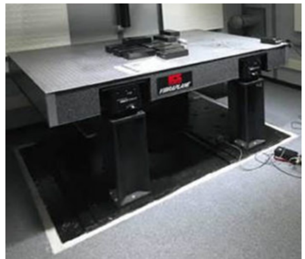
Customized Minus K Technology Negative-Stiffness vibration isolation table installed in the Ultra-Low Vibration Lab.
