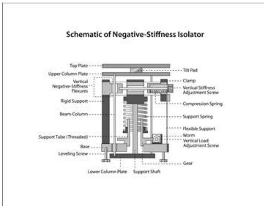
*Schematic of a Negative-Stiffness isolator.*
