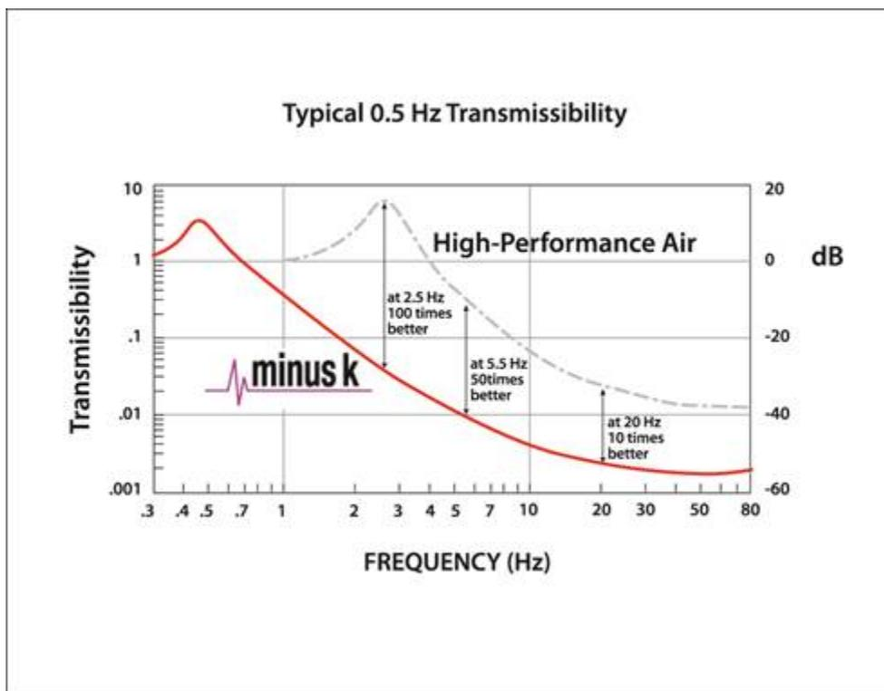
*Vibration transmissibility compared, Negative-Stiffness compared to air tables.*
