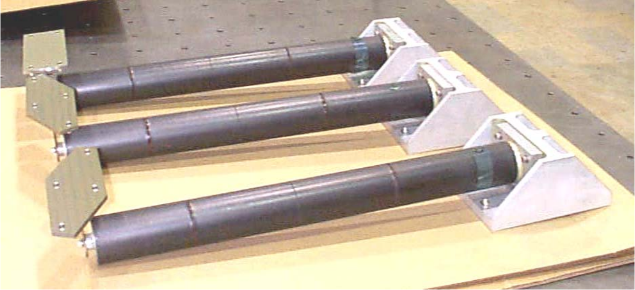
Figure 4. Backpack Isolator Struts Prior to Installation
